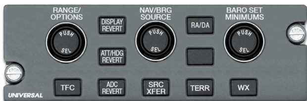
PFD Combined Display Control Panel
