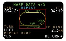
Airdrop Data Page 4 displays navigation information relating to the loaded airdrop profile including repeat pattern flight path data.
