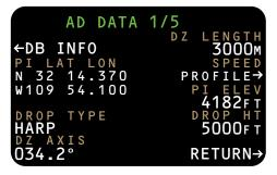
On Data Page 1, the operator can enter Point of Impact location, aircraft speed profiles related to the Air Release Point, and edit other drop profile parameters.
