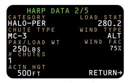
Airdrop Data Page 2 displays information for the selected type of airdrop including chute data, load parameters, and wind considerations.
